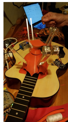
(b) Pico Robot (2nd gen). Mechanical arms strike tuning forks on a guitar body.
