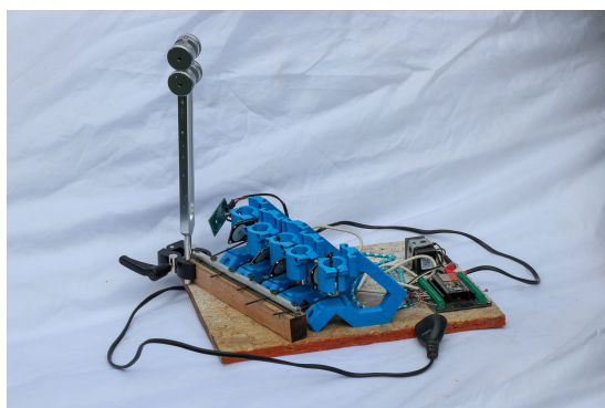
(c) Beacon 3 (3rd gen). Piezoelectric motors drive metal reeds, controlled wirelessly via Bluetooth from a 64-pad harmonic surface.
