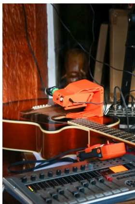
(a) Beacon Guitar (1st gen). Motor-driven string coupled to acoustic body.
